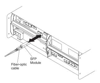
Figure 8. SFP module and fiber-optic cable
